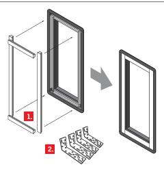
Replacement kit for all sizes of VS and most FS\* skylights. Allows the installer to use a standard size VELUX VS or FS skylight on a non-standard opening while minimizing the amount of interior trim work needed.
